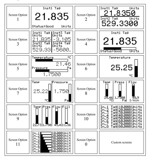
Setting the "*Screen Option"* Modbus register to a value of 0 will allow custom screens to be displayed by using BEKA protocol commands.
